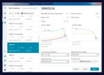
STS tool: Easy input of motor and load data
